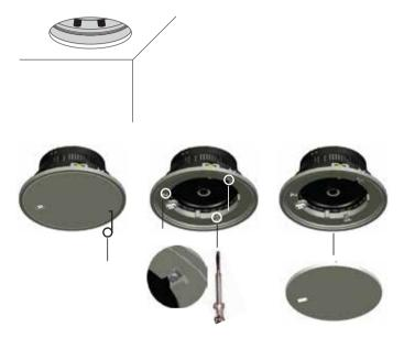
(ENG) installation in false ceiling (depth 85mm)
