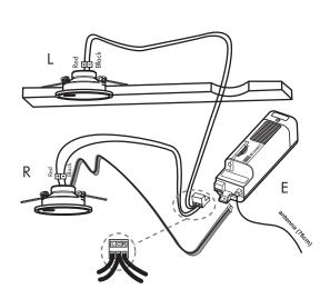
Connect loudspeakers R and L to connecting terminals L, C and R on the electronic module E.
