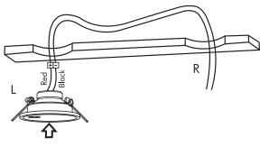
Insert loudspeaker L and pull the joining cables to the other loudspeakers R's location.
