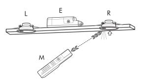
Insert the electronic module  $\ensuremath{\mathsf{E}}$  through the cavity prepared for loudspeaker R. Make sure the antenna cable is not near to possible noise sources such as fluorescent bulbs, power supplies, halogen lamps, fans, motors, etc. which could hamper the radio station reception and affect sound quality.
